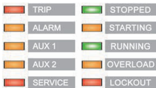
FIGURE 4-1: LED Indicators - Enhanced Faceplate
