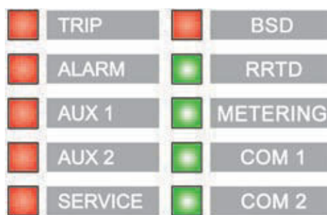
FIGURE 4-2: LED Indicators - Basic Faceplate
